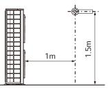
1. These figures assume the following operating conditions : Equivalent piping length : 7.5m Level difference : 0m
