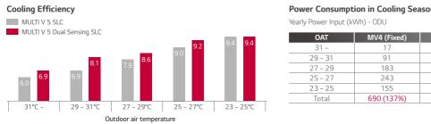
% This energy simulation was performed in LG internally based on 16HP model.
