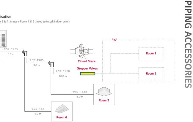
• In case of installation of additional indoor unit, refrigerant of used indoor unit must be discharged. (Room 3 & Room 4) • If stopper valve is already installed, you can install additional indoor unit without refrigerant loss from the entire system. • After installation of additional indoor unit, you just need refrigerant charging for "A" section. • Then, open the Stopper Valve.
