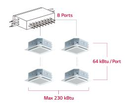
Flexible Connection Series connection can be installed without pipes crossing.
