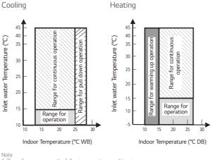
Note 1. These figures assume the following operating conditions: 2. Equivalent piping length :7.5m 3. Level difference : Om
