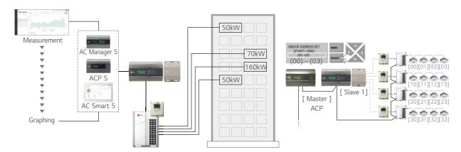
Note : 1. Power cable and type could be different from this scene depending on the Outdoor unit's specification. 2. Measured power consumption could be different between PDI and Watt meter. 3. Applicable Central Controller : ACP 5, ACP LonWorks, AC Smart 5, AC Ez Touch (Combination : we recommend to connect separated watt meter for Outdoor units to have correct power distribution value)
