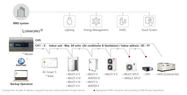
PI485 converts LG Air conditioners protocol to the RS485 protocol for the central controller.
