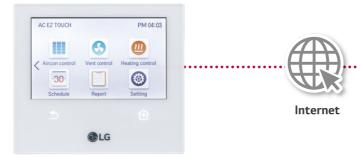
\* IPv6 supported - Open port 80 & 9300 - Fix public IP is mandatory. Router configuration of NAT is required.
