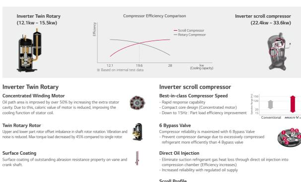
Scroll Profile - The enhanced reliability by Increased reliability with regulated oil supply - Efficiency increases by expanding 96% Bypass area and 17% improved volume ratio by non-uniform scroll thickness
