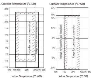
1. These figures assume the following operating conditions Equivalent piping length : 7.5m Level difference : Om
