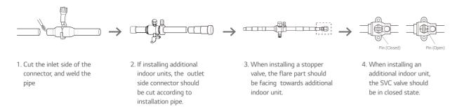
% When welding, service valve should be wrapped by wet cloth.
