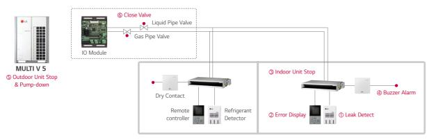
\* If the concentration of the refrigerant in the air exceeds 6,000 ppm more than 5 seconds, the function will be activated. (Refer to operation sequence which written in red, 1-6)
