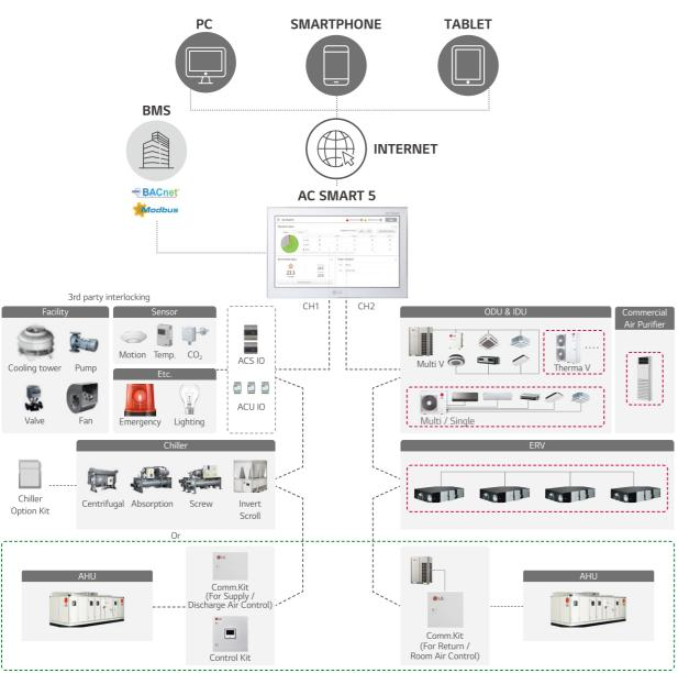
C According to CH1 setting, normal ODU can be connected to CH1.
