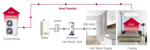
HYDRO KIT Absorbed heat from indoor space is used for making hot water.
