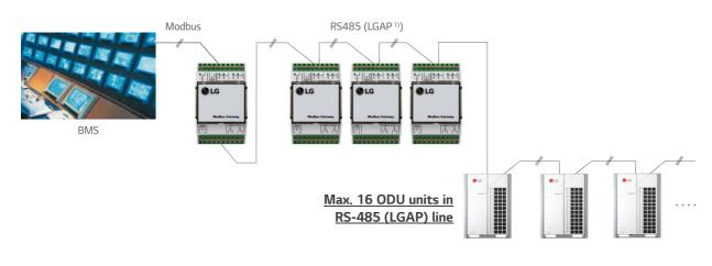
1) LGAP is LG Protocol. Max. 16 ODU units in RS-485
