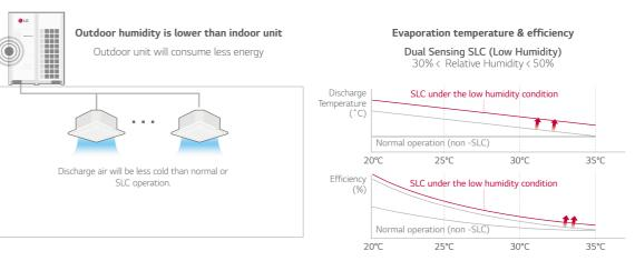
To maximize comfort and energy efficiency, the outdoor unit's humidity sensing can be turned off or a standard remote control can be installed to sense indoor humidity.
