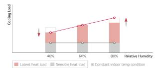
Cooling load according to humidity change
