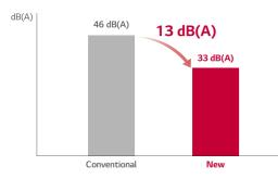
Test Condition (ISO Standard) - Temp.: (Cooling) 27℃ DB / 19℃ WB, 35℃ DB / 24℃ WB (Heating) 20℃ DB / 15℃ WB, 7℃ DB / 6℃ WB - Operating : cooling → heating switching operation
