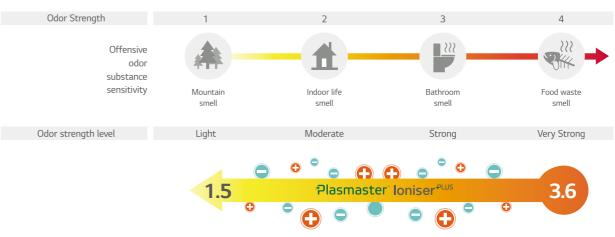
Odor strength reduce 3.6  $\Rightarrow$  1.5 / The Odor floating in the room as well as curtain and clothes. ※ Test conditions : Space: 8m<sup>3</sup> Chamber Temperature & Humidify : Normal Tested by Intertek
