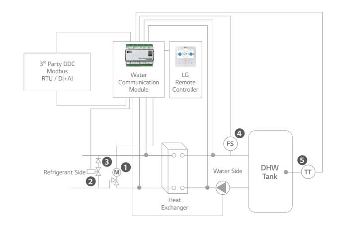
• 3rd party solenoid, non-return valve, heat exchanger, flow switch and DHW temperature transmitter (Optional) must be purchased separately. (Field supplied items)
