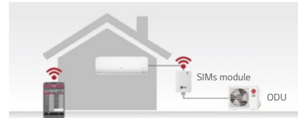
* SIMs : Smart Inverter Monitoring System
