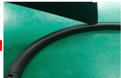
Insert the tool to the edge, and then disassemble from left to right .
