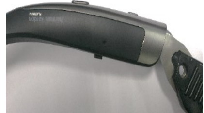
Insert the tool to the edge, and then disassemble from right to left .
