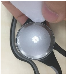
Using a tool, detach Upper case.
