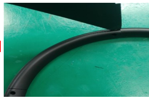
Insert the tool to the edge, and then disassemble from left to right .
