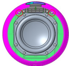
4) Disassemble of the Jersey Assy (2 screw)
