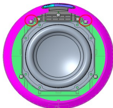
3) Disassemble of the Jersey Assy (2 screw)
