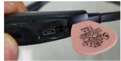
Insert the tool to the edge, and then disassemble from right to left.
