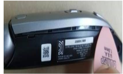
Insert the tool to the edge, and then disassemble from right to left.
