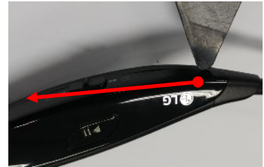
Insert the tool to the edge, and then disassemble from right to left.
