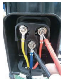
Measuring resistance between each terminal of compressor
